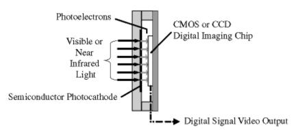
When light photons strike the photocathode, electrons are emitted. High voltage between the photocathode and imaging chip accelerates the electrons across a vacuum gap onto the imaging chip, which then produces an amplified digital signal.
