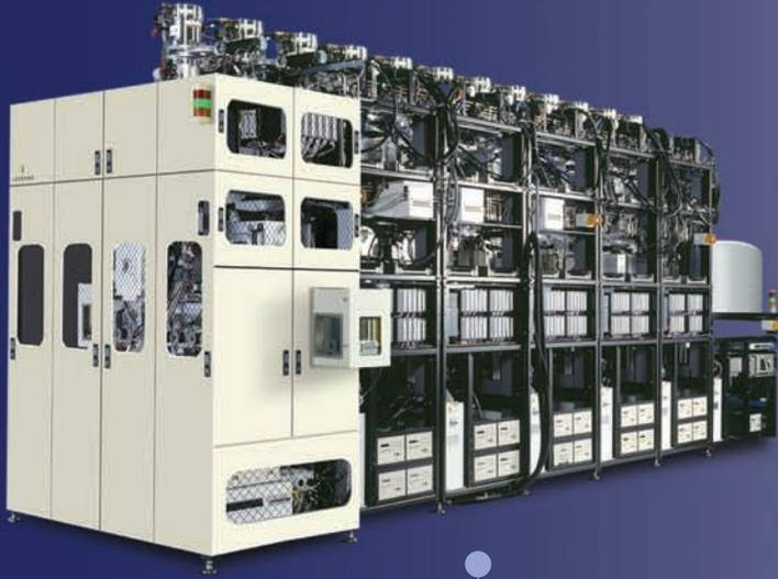
The 200 Lean magnetic media deposition system is used by disk media manufacturers worldwide and has an installed base of over 110 systems.
